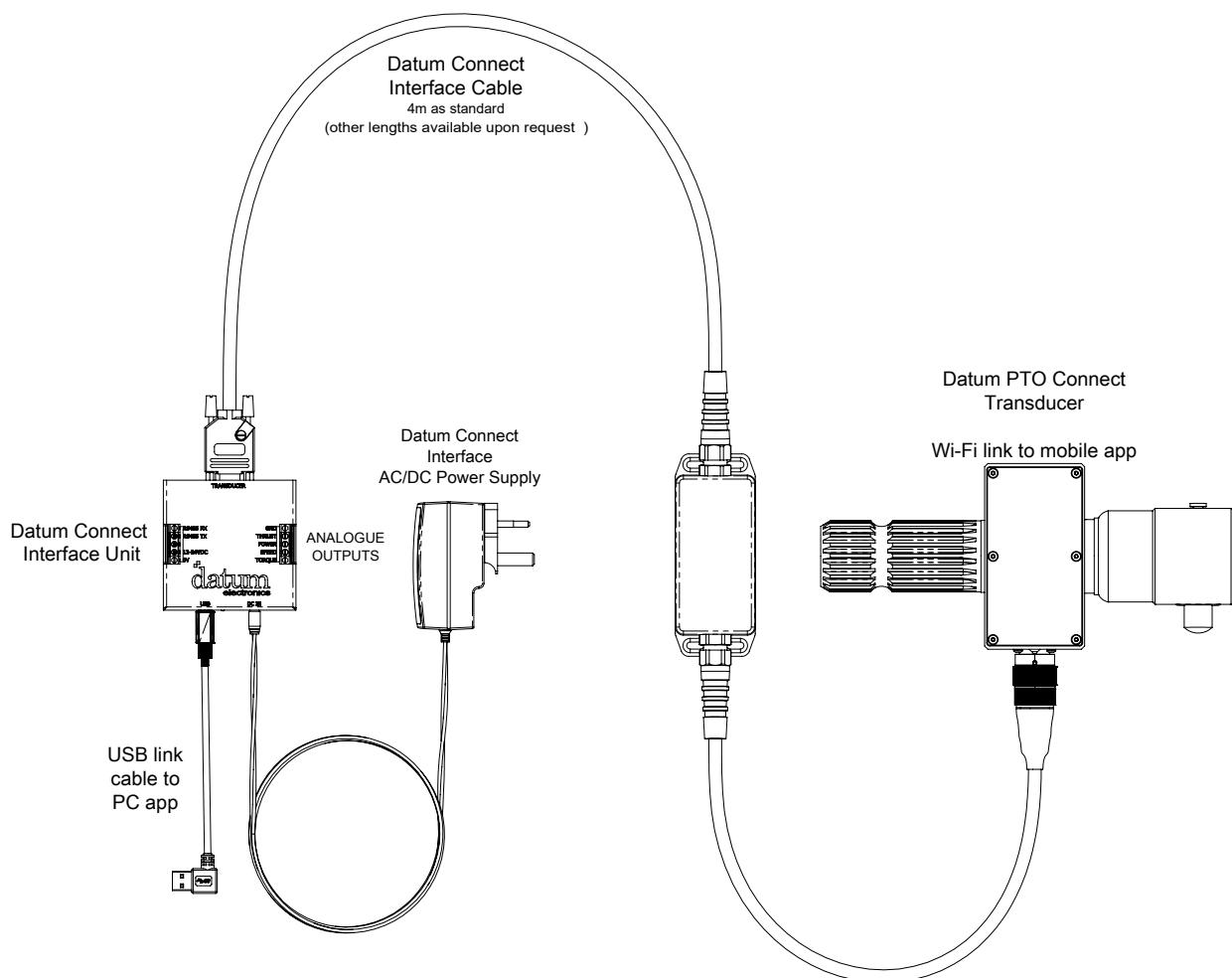
For applications other than the one shown above please contact Datum Electronics for power supply requirements (including DC supply options)
