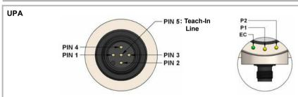
EC (Echo LED) green: is on, when an echo is received (alignment LED).
