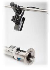
The system is designed for measuring power and torque on drive shafts, applications including marine ship shafts, prop shafts and vehicle drive shafts. The trials kit measures the on-shaft torque and wirelessly sends this data to the off shaft receiver which is also the optic speed sensor. The data is outputted via USB to a laptop/netbook to our free software, PowerKit. The Torque, Speed and Power can then be viewed or logged as required
