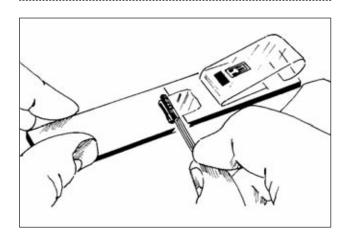
Coat the specimen, back of the gauge, and terminal strip with the prepared adhesive. The mixing rod can be used to apply a thin layer of adhesive over each surface. Be careful not to pick up any unmixed components of the adhesive. To ensure this, it is advisable to wipe the mixing rod clean and then pick up a very small amount of the adhesive from the center area of the adhesive jar.
