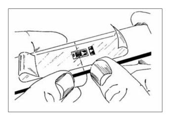
Position the gauge/tape assembly so the triangle alignment marks on the gauge are over the layout lines on the specimen. Holding the tape at a shallow angle, wipe the assembly onto the specimen surface. If the assembly appears to be misaligned, lift one end of the tape at a shallow angle until the assembly is free of the specimen.
