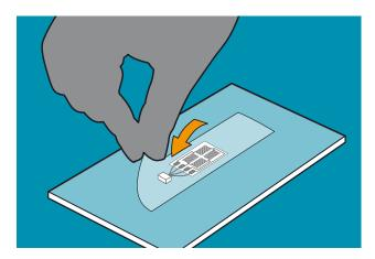
3. Cut a length of mylar tape approximately 150mm in length. Carefully offer the tape to the top side of the gauge and stick the gauge roughly in the centre of the mylar tape (see above). Stick the tape onto the glass plate with the gauge in a central position.
