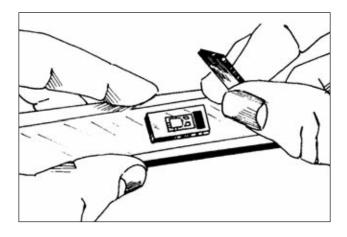
Place a silicone gum pad and backup plate (GT-14) over the gauge installation. The silicone gum should be soft (Durometer A40-60) and at least 3/32 in [2.5 mm] thick. This will allow the clamping force to be exerted evenly over the gauge. The area of the silicone gum pad should be used to compute the final clamping pressure.
