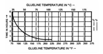
Caution: These systems may not cure properly below  $+70^{\circ}F$  [ $+20^{\circ}C$ ]. Postcuring the installation for two hours at least  $+25^{\circ}F$  [ $+15^{\circ}C$ ] above the maximum operating temperature with the clamping fixture removed will provide essentially creep-free performance.
