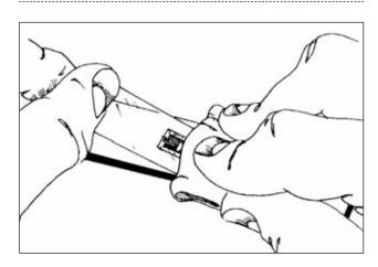
Immediately rotate the tape to approximately a 30-degree angle so that the gauge is bridged over the installation area. While holding the tape slightly taut, slowly and firmly make a single wiping stroke over the gauge/tape assembly with a piece of gauze bringing the gauge back down over the alignment marks on the specimen. Use a firm pressure with your fingers when wiping over the gauge. A very thin, uniform layer of adhesive is desired for optimum bond performance.
