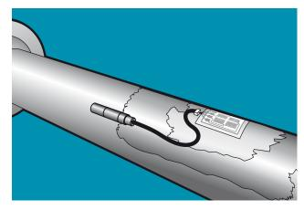
Apply pressure to the edges of the Teflon tape to provide a good seal around the gauge.
