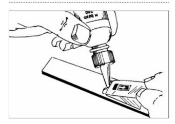
Lift the tucked-under tape end of the assembly, and, holding in the same position, apply one or two drops of MBond 200 adhesive at the fold formed by the junction of the tape and specimen surface. This adhesive application should be approximately 1/2 in [13 mm] outside the actual gauge installation area. This will insure that local polymerization that takes place when the adhesive comes in contact with the specimen surface will not cause unevenness in the gauge glueline.
