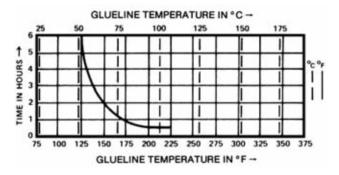
Caution: To ensure proper polymerization, the cure cycle should start within 1.5 hours after mixing.
