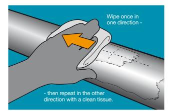
12. When neutralised, the surface should be dried by wiping across the cleaned area with a single slow stroke of a clean lint-free tissue. With a fresh lint-free tissue, a single stroke should then be made in the opposite direction, beginning within the cleaned area and moving outwards to avoid recontamination from the uncleaned boundary (see above).
