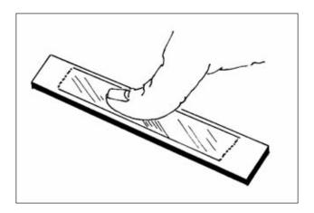
Immediately upon completion of wipe-out of the adhesive, firm thumb pressure must be applied to the gauge and terminal area. This pressure should be held for at least one minute. In low-humidity conditions (below 30%), or if the ambient temperature is below  $+70^{\circ}$ F [ $+20^{\circ}$ C], this pressure application time may have to be extended to several minutes.
