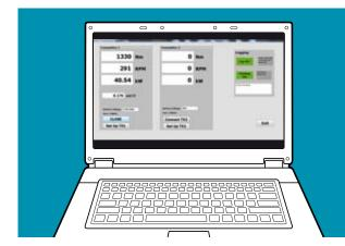
3. Once the gauge is installed, and with either a handheld indicator or PC connected, you should if possible apply a twist to the shaft. Applying a small torque to the shaft by hand or by a manual lever is usually sufficient to allow you to see the readings on the display change. By applying a small force in this way you are able to gain additional confidence in your strain gauge installation.
