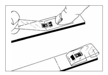
Lift one end of the tape at a shallow angle to surface (about 45 degrees) until gauge and terminal are free of specimen surface. Tuck the loose end of the tape under and press to the surface so the gauge lies flat with the bonding side exposed. In some cases this may be difficult because of space limitations. If this situation occurs, leave enough slack in the tape to allow a finger to be slipped behind the gauge to support it while applying the adhesive.
