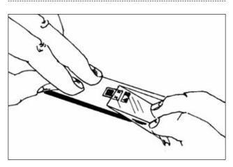
The gauge and terminal strip are now solidly bonded in place. It is not necessary to remove the tape immediately after gauge installation. The tape will offer mechanical protection for the grid surface and may be left in place until it is removed for gauge wiring. To remove the tape, pull it back directly over itself, peeling it slowly and steadily off the surface. This technique will prevent possible lifting of the foil on open-faced gauges or other damage to the installation.
