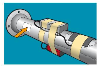
2. Cut a piece of reflective tape approximately 30mm x 100mm and position it on the shaft.
