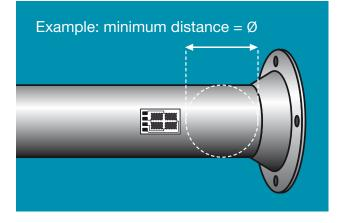
2. Measure the diameter of the shaft. The gauging area should be no less than one shaft diameter away from any obstruction or shaft joint (see above).
