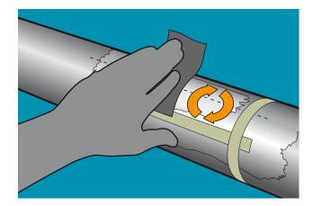
Second stage abrading uses silicon carbon paper of the appropriate grit. It is recommended that abrading should start at 120 grit progressing through to 400 grit in a random pattern to attain a flat, clean, and well keyed surface (see above).
