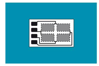
The strain gauge supplied by Datum Electronics is a full bridge encapsulated gauge complete with a connector. These simplify the installation process and remove the need for soldering on site. The gauge has fine elements within its grid that measure strain. These elements can be seen under a magnifier and should be aligned at 45 degrees to the axis of the shaft to measure the torsional strain.
