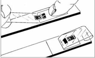
Lift the gauge end of the tape assembly at a shallow angle to the specimen surface (about 45 degrees) until the gauge and terminal are free of the specimen surface. Continue lifting the tape until it is free from the specimen approximately 1/2 in [10 mm] beyond the terminal. Tuck the loose end of the tape under and press to the specimen surface so that the gauge and terminal lie flat, with the bonding surface exposed.
