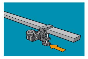
1. Attach the Receiver Mounting Clamp to the suitable structure and tighten the locking wheels (see above).
