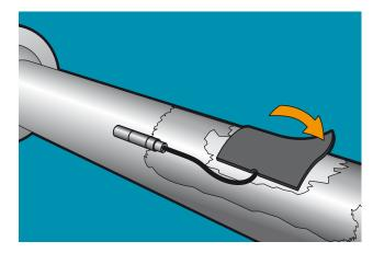
3. Cut a strip of butyl mastic large enough to cover the strain gauge and the area of Teflon, and stick over gauge onto the cleaned area where the strain gauge is bonded to the shaft (see above). Apply pressure to the edges of the mastic to provide a good seal around the gauging area but leave the cable exposed. The shaft area needs to be chemically clean for the mastic to adhere - warming the mastic to 25-30°C will also assist with fitting and adhesion.
