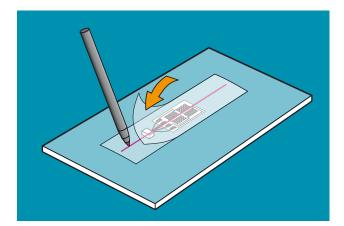
4. After applying the first layer of tape mark a line across the gauge (see above) using an indelible marker, parallel to the long side of the gauge. Then add a second layer of mylar tape. The second layer will stop the tape curling when applying the gauge to the shaft.
