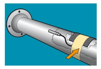
4. At higher revolutions additional layers of cross weave tape should be used to secure the mastic coatings. Suitable tapes to use are either Strong Cross Weave Tape or and Adhesive Glass Cloth Tape with a strength in excess of 25kgs per cm.
