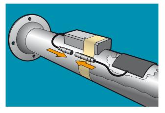
2. Plug the strain gauge connector into Transmitter connector. Wrap excess cable around Transmitter Enclosure.
