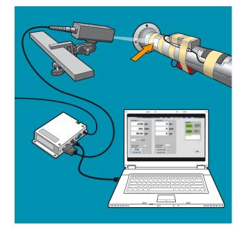
The cable run from the Receiver to the Interface should be secured approximately every 0.5 metres so as not to become a hazard. IMPORTANT NOTE: When running cable ensure that it is not mounted in any area that may become damaged by the moving or rotational machinery. Coil up and securely tie any excess cable.
