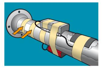
3. Hold it in place by wrapping tape around the shaft at each end of the reflective tape.
