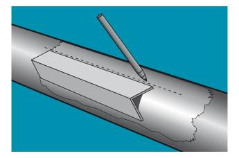
3. Place the angled bar flush to the shaft, and mark a line parallel to the shaft using a ball point pen (see above). This will act as a burnished line positioning guide to the centre line you marked on the mylar tape over the gauge in Stage 1.4.
