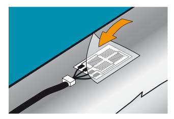
1. Cut a piece of Teflon tape (approx 30mm long) to cover the gauge and the connector, and stick it over the strain gauge onto the cleaned area where the strain gauge is bonded to the shaft.
