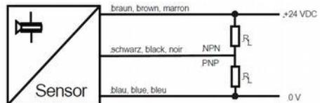
**UX micro 500-PS-24-C-SY** PNP NO, 4 pole connector, synchronisation input
