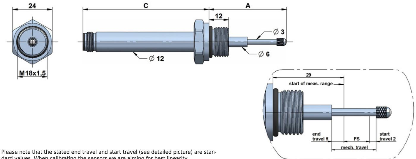
Please note that the stated end travel and start travel (see detailed picture) are standard values. When calibrating the sensors we are aiming for best linearity.
