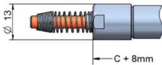
Sensors with cable output have a cable fitting and a spring for bend protection of the cable.
