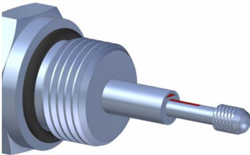
The option VH should be chosen, if the sensor is used in liquids (oil, water, ...) or if fast pressure variations may occur. By milling plane surfaces on parts of the mechanics (see picture red marked) the pressure balance or venting of the inside area will be improved.
