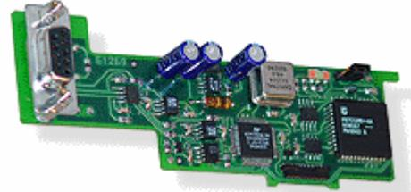
The PAX PROFIBUS-DP Communications Option Card provides a direct connection for a PAX panel meter to a PROFIBUS-DP Network. This allows a PROFIBUS Master device, such as a PLC, to control and monitor the operation of the PAX meter. The meter functions as an intelligent PROFIBUS-DP Slave device on the Network.
