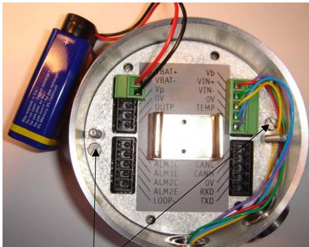
Loosen screws to change display orientation.
