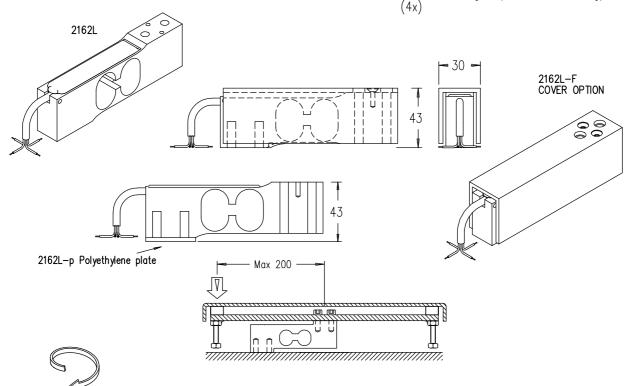
Note:Correct torque for fixing bolts : 10 Nm if M8 50 Nm if M10 (don't touch bottom of tapped holes)
