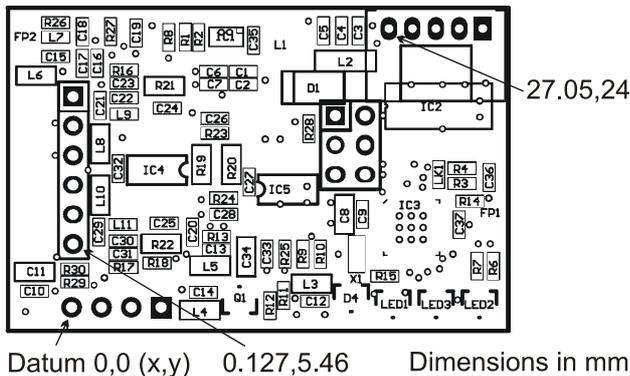
The PCB can be fitted to a motherboard by fitting in-line pins to the 6-way, 4-way and 5-way rows of holes and plugging them into corresponding sockets on the motherboard or directly soldering through holes. The 6-way and 4-way holes are on a 0.1" pitch, the 5-way holes are on a 2mm pitch.
