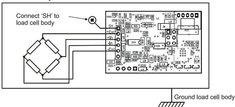
If the DCell is mounted outside the body of the load cell then, for optimal performance, twin twisted cable should be used, although standard 4 core shielded cable can be used in **low** noise environments.
