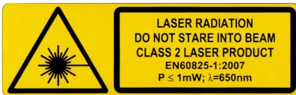
Figure 2 : Warning Sign Laser Radiation Class 2
