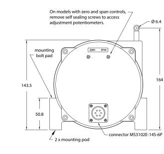
Note: Sensor mounts with M12 cylinder head screws.
