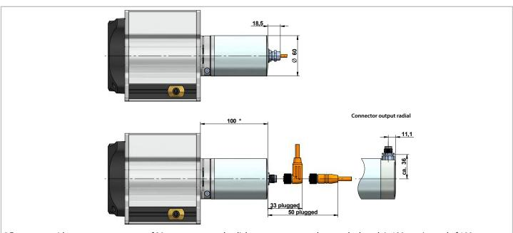
\* For sensors with measurement ranges of 30 m or greater and radial connector output the encoder length is 120 mm instead of 100 mm.
