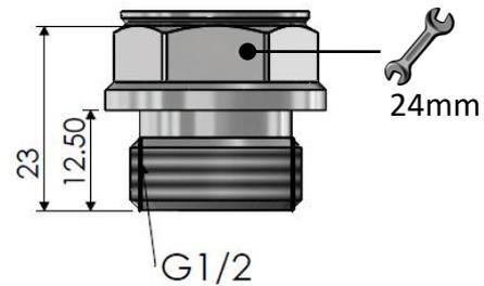
\* In the case of the G1/2 model, the dimension of key slot is 24mm. All other models are 22mm.
